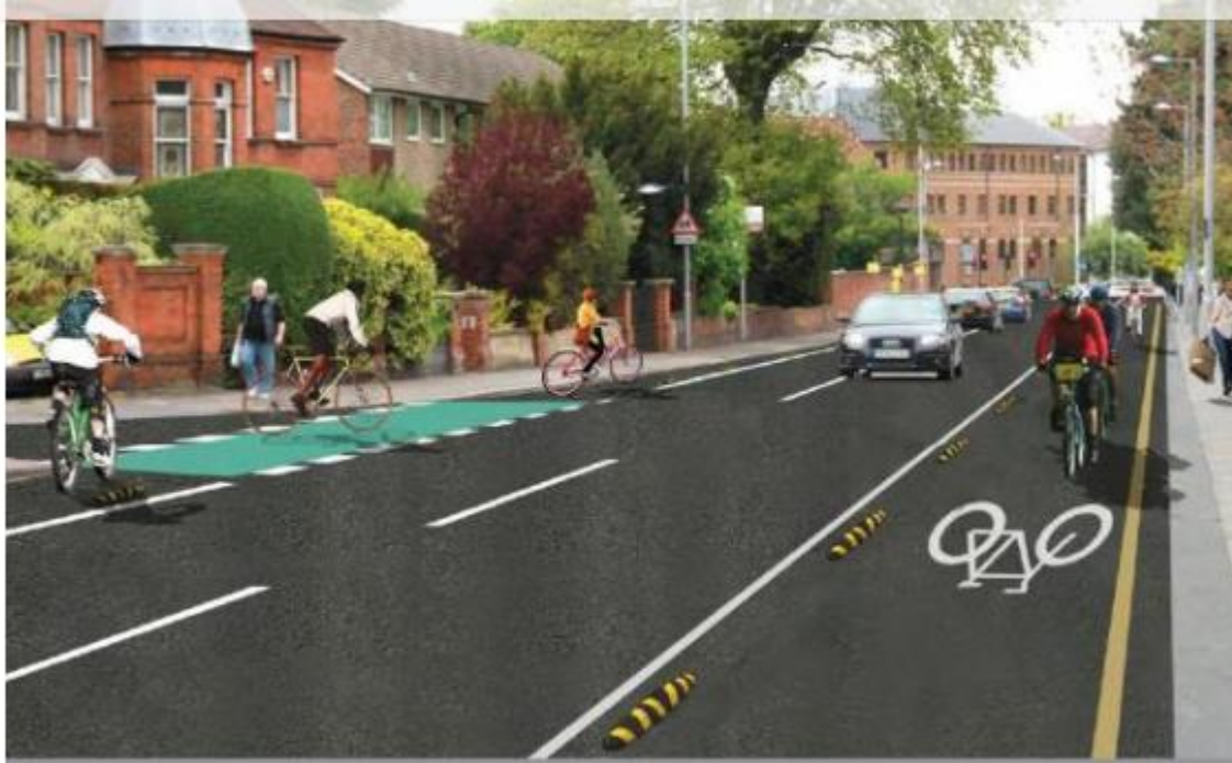
Dedicated widened cycle lanes on carriage with delineating “armadillos” to restrict vehicle ingress (Marton/Acklam/Ormesby/Cargo Fleet Roads – main corridors)
